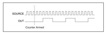
Figure 7-25. Continuous Pulse Train Generation
